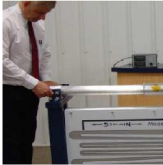
*Tighten block end knobs fully. Then tighten red yoke knobs securely.*
