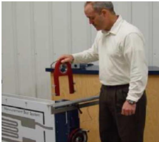
Loosen capture knobs, remove yoke.
