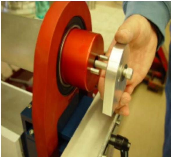
*Insert Cantilever Load Block on red end.*
