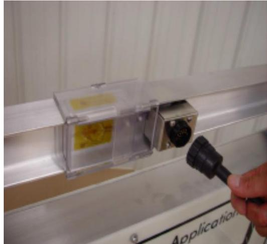
*Plug in Data Box Multi-Pin Connector.*
