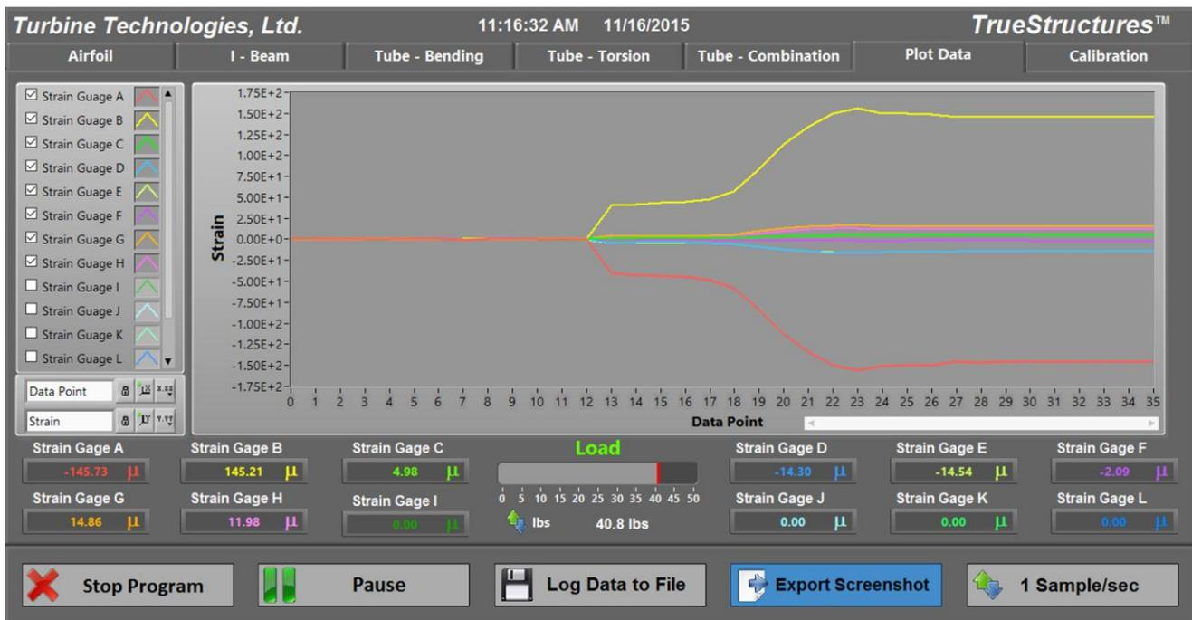
Torsion Tube Pure Bending Strain Plot Data Screen
