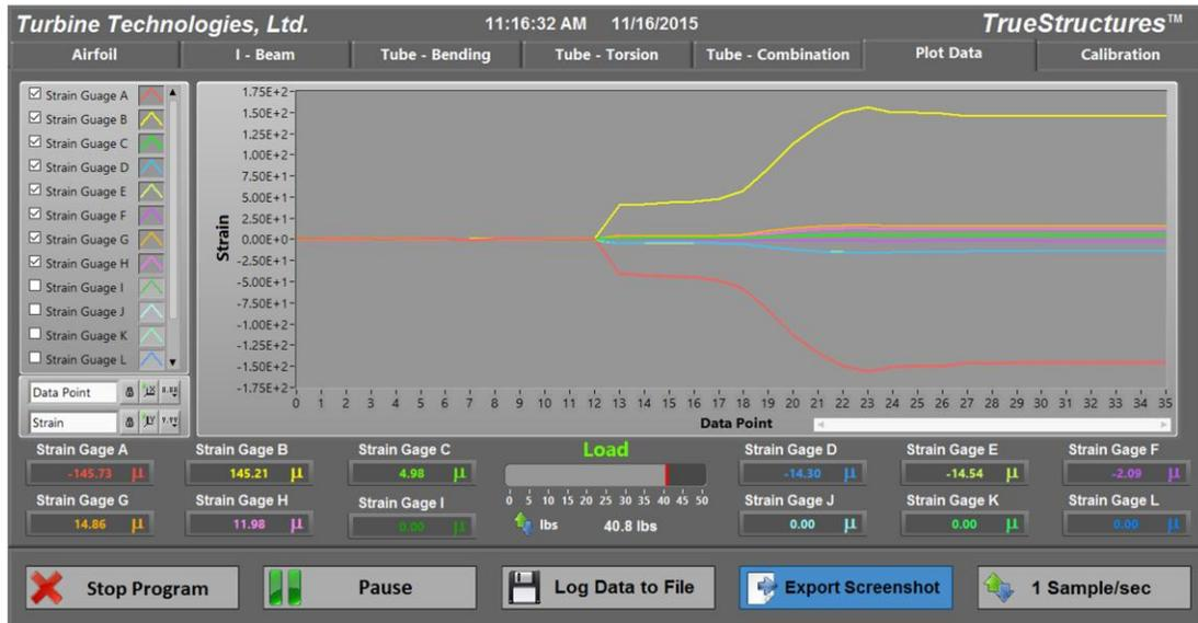
*Torsion Tube Pure Bending Strain Plot Data*
