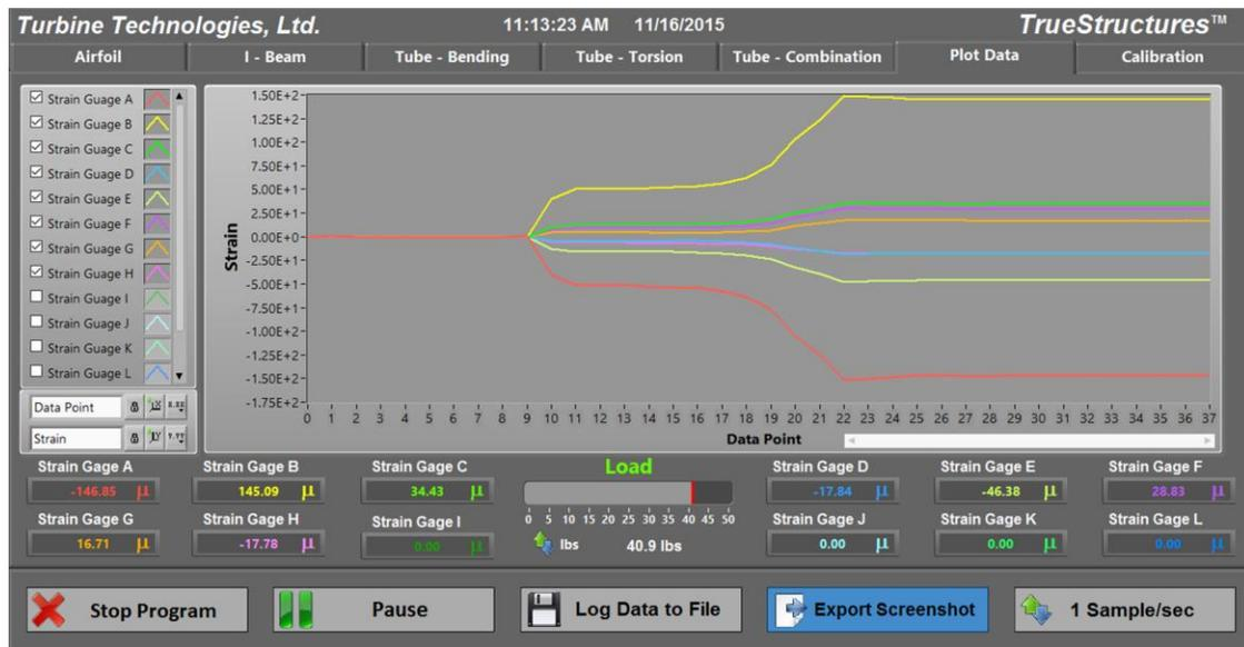
*Torsion Tube Combination Loading Data Plot Screen*
