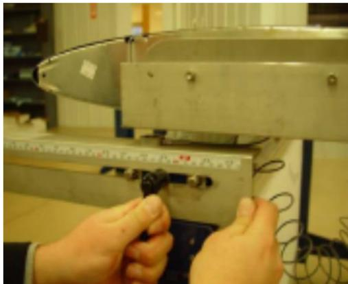
*Loosen friction lock to position load cell.*
