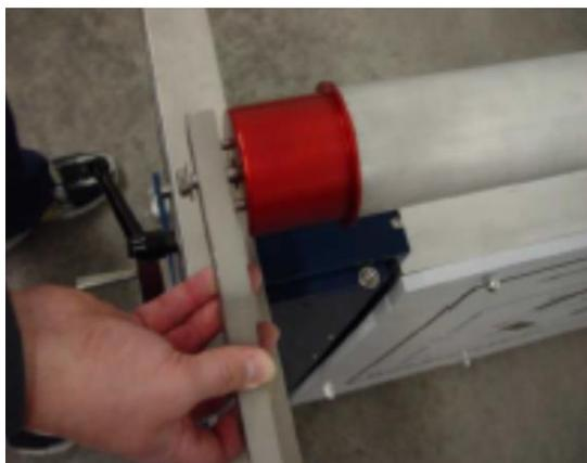
Insert Torque Arm into Tube End.
