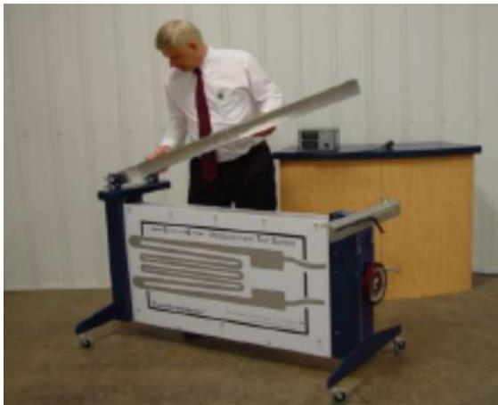
*Position I-Beam Assembly onto Frame*
