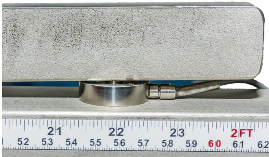
*Load Cell under Torque Arm*
