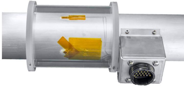
*Torsion Tube Strain Gage Layout with Multi-Pin Connection Box*
