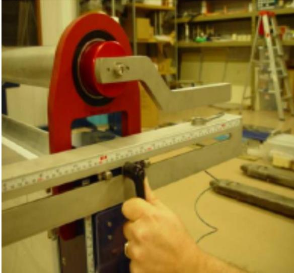
*Position Load Cell to desired moment arm dimension from tube centerline (Step 2).*
