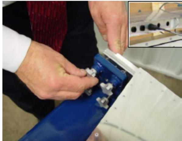
*Finger-tighten knobs. Lift up on cantilever end of wing to remove any sag in system. Tighten knobs firmly while continuing to lift end of wing.*
