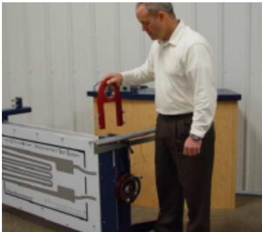
*Position Yoke on Crank End (note correct face out as marked)*
