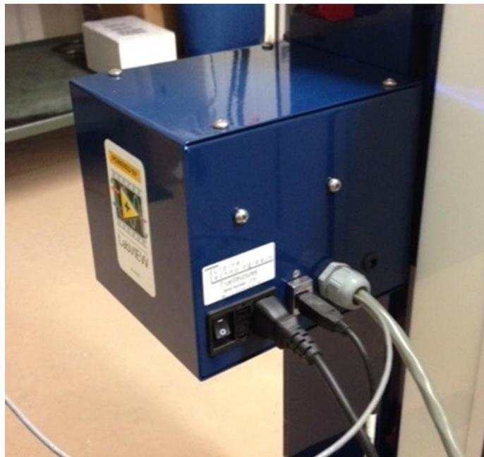
*Connections into Data Acquisition Box*
