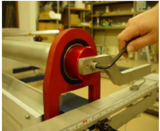
*Tighten Torque Arm Bolt securely with Allen Wrench.*
